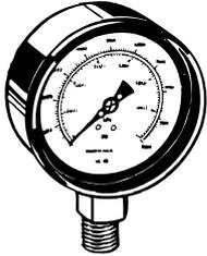
All hydraulic systems should have a gauge. The gauge is the window to the hydraulic system. In addition to indicating the operating pressure, the gauge can also warn you that something is going wrong.
