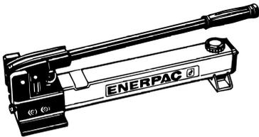
Hand pumps are a convenient, portable source of hydraulic power. They are designed to be stable during operation. For best performance, operate the pump handle at moderate speed. When the handle gets hard to push at high pressure, take short strokes. The maximum leverage is obtained in the last 5 degrees of stroke. Adding an extension dangerous.
