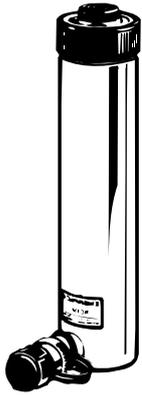
The saddle in the plunger serves two important purposes. It protects the plunger threads from damage and it keeps the end of the plunger from becoming deformed. Keep the saddle in place at all times. Do not thread attachments into the plunger and rely on the plunger threads for support. The load must be transferred to the face of the plunger. The threads in the plunger may be stripped if loaded.
