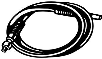
Rubber hoses are made in 4 layers: a rubber tube on the inside, 2 layers of wire braid, and a protective rubber layer on the outside. If the wire braid can be seen from the outside, it is time to replace the hose. Rubber hoses have a 2:1 safety factor. Thermoplastic hoses are frequently used with power-driven hydraulic pumps. Only 700 series thermoplastic hoses have a 4:1 safety factor.
